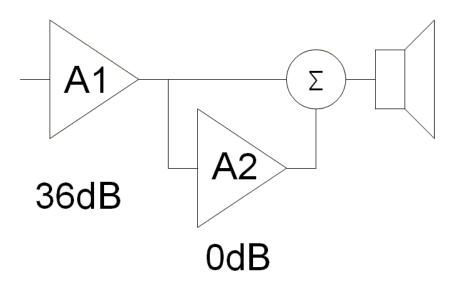
The Tube amplifier provides all the Voltage gain and a certain amount of the total current to speaker.
